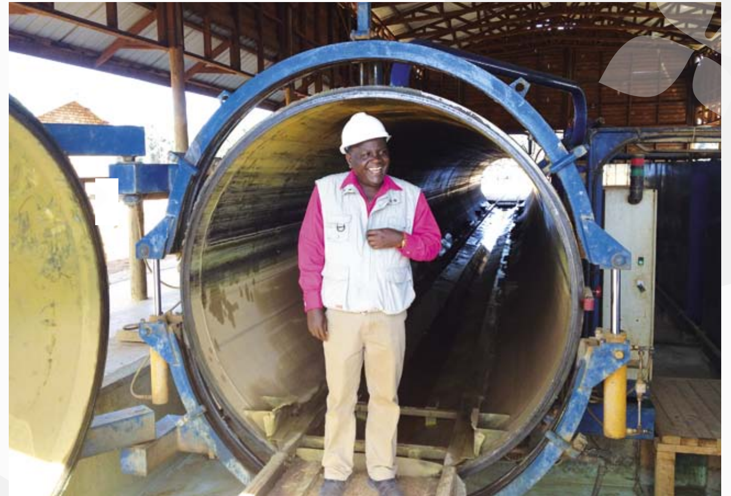
Mr Martin Kawonga at a machine for impregnating poles at Green Resource's forestry operations in Sao Hill, Tanzania.
